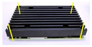
6. Use M2.5 screws to fix the heatsink together with module.
