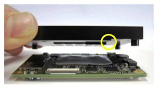
5. Mount the heatsink in a way that the position of the holes is right from the beginning (moving it may not be possible since the TIM sticks the aluminium and print together).
