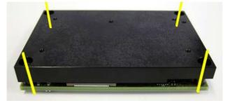
6. Use M2.5 screws to fix the heatsink together with module.
