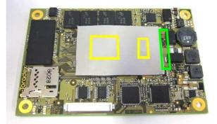
4. On attaching the heatsink, make sure the yellow marked corner is on the right side. (Very important for Robin since she position of the screws don't assure that it is mounted correctly).
