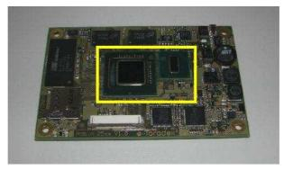
2. Remove the plastic foils on the TIM (on both sides) and attach the TIM as shown over the SCH and CPU.
