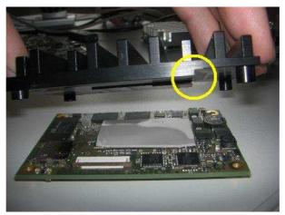
5. Mount the heatsink in a way that the position of the holes is right from the beginning (moving it may not be possible since the TIM sticks the aluminium and print together).
