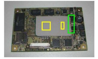
4. On attaching the heatsink, make sure the yellow marked corner is on the right side. (Very important for Robin since she position of the screws don't assure that it is mounted correctly).
